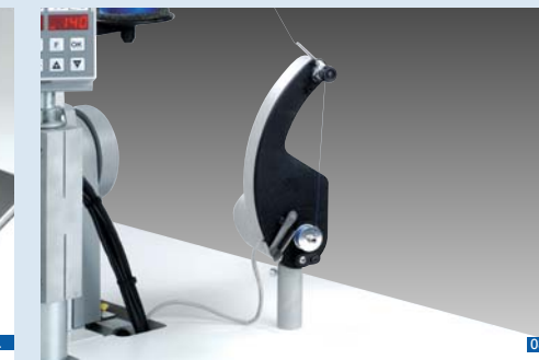
External bobbin winder • Separately driven bobbin winder for rapid colour change.
