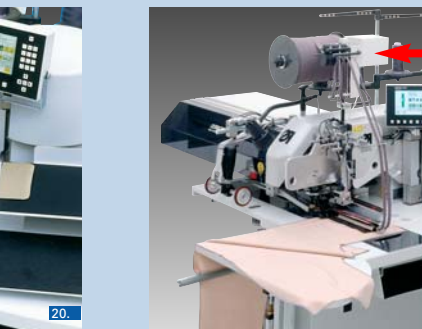
Device for endless zippers • Includes zipper scissors with unwinding device for displacement-free attaching of endless zippers without slider. Optionally one zipper feeder (0793 026561 or 0793 026021) has to be ordered. The device is to be used in conjunction with E2607 (for other equipment on enquiry).
