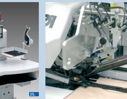
Zipper feeder for endless zippers without slider • In conjunction with device 0745 597544 and folder S100 (0793 026503). This working method allows to add pocket bag halves as well. Note: When ordering please enclose zipper samples for adaptation of the feeder.
