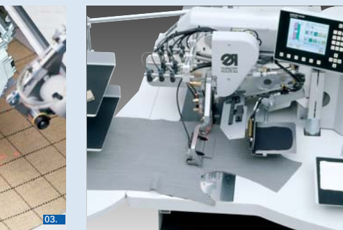
Class 745-34D • Matching and feeding device for breast welts and pocket bags • Free view of the working area for the precise positioning of chequered and striped breast welts. Previous marking of the breast welts is not required.
