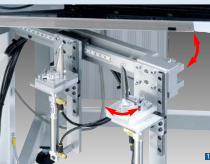
Mechanically adjustable corner knife station • Corner knife station for straight pocket openings with easily adjustable corner incision system; the incision angle can individually be adjusted mechanically; the corner knife station can be swivelled out for adjustment purposes (class 745-34S).
