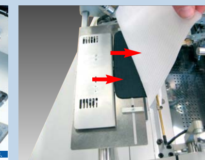
Set of parts "Pocket bag on flap" • For the simultaneous attaching of two pocket bag halves and the flap in one operation. Through this, considerable increase in productivity will be achieved in the manufacturing of men's jackets (only in conjunction with the equipments E03103, E03503, E03107 or E03507).
