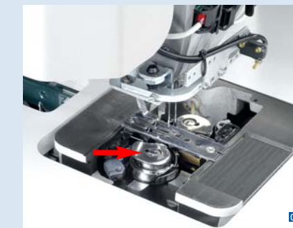
Large hook • Vertical hook for large bobbin capacity.
