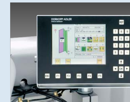
Control panel with coloured graphic display • Large coloured graphic display with individually adaptable user interface, with symbols and explaining texts; 99 sewing programs and 20 sequences can be memorized; up to 8 programs can be stored in one sequence.
